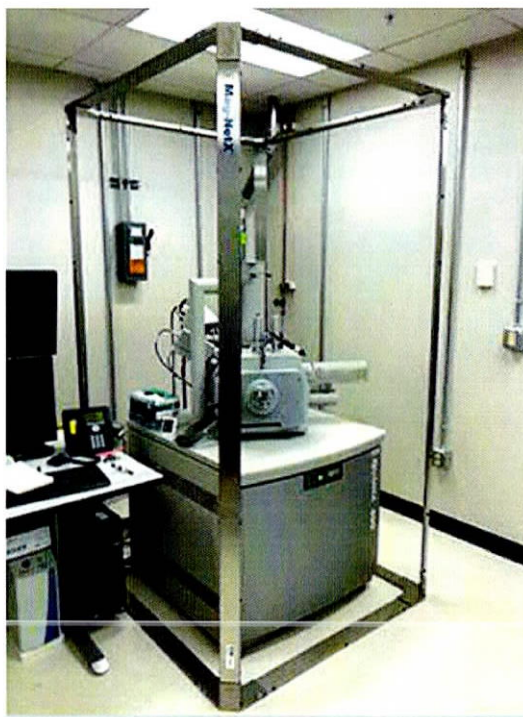
Figure 8: Mag-NetX Active Magnetic Field Cancellation system [15]
